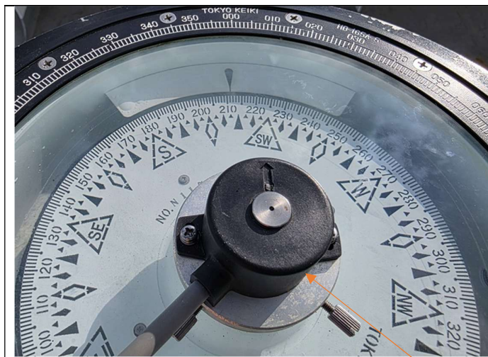
Ship's magnetic heading on compass card, sensor converts the magnetic compass heading to electrical signal
